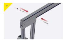
> Insert and tighten the final beam bolt
