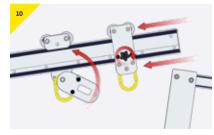
Thread the beam trolley over the other end of the beam and lock with the friction brake at approximately centre position. If using a gated trolley, lock with the friction break
