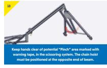
With the help of another person, scissor the beam and A-Frame into position (using the first bolt as a hinge). Be careful not to trap any fingers in this operation
