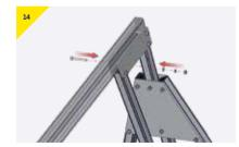
Insert the second bolt into the cheek-plate. Tighten both bolts until spring washer is fully depressed, be cautious not to overtighten
