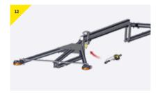
At this stage it is useful to attach the lifting device to the trolley in order to avoid having to lift and attach when gantry is fully erect. This avoids a working at height problem when attaching a hoist
