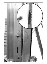
When the brake is engaged, it will be possible to see the Brake Cam acting on the adjacent mast section.
