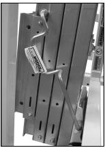
The winch handles have been placed in the stored position.
