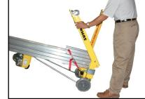
While holding the leg in the 90 degree position, slide the Leg Lock back towards the leg until the spring loaded plunger pin engages into position.
