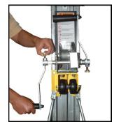
up on the locking pin and slide the handle off of the winch shaft. Rotate the handle assembly around so that the black plastic grip is facing away from the winch. While pulling up on the locking pin, slide the handle back on to the winch shaft. Repeat this procedure for the other handle.
