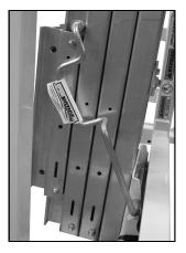
To release Hold Down, pull bar toward you and place back behind mast sections.
