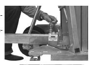
Unlock caster swivel lock on cart to allow rear caster to swivel freely during operation.
