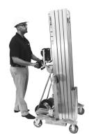
The Counter Weight Cart can be rocked back on it's 8" wheels and transported like a dolly. Be sure to engage caster lock so that caster may not swivel.
