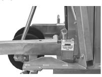
This condition can be corrected using the adjustment knob. First, loosen the lock nut located in the saddle. Turn the large adjustment knob counter clockwise to raise the
