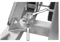
saddle and clock wise to lower the saddle. Once the saddle is level with the Extension Leg re-tighten the lock nut.
