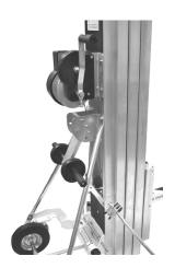
Turn winch crank clockwise to elevate the load, while watching for overhead obstructions.
