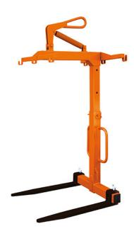
The 1055T has been designed to give flexibility when required to move oversized and normal packs of block and brick s as well as palletised goods around site. This unit is supplied with heavy duty sprung lifting eye allowing automatic levelling of any load being carried. The unit also comes supplied with net hooks allowing the addition of a load safety net
